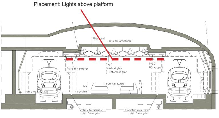
Design & Placement: Working Light & Fixture
